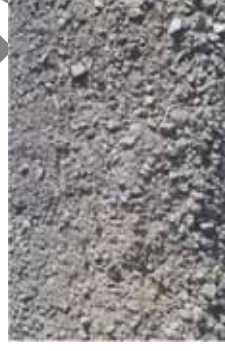
DOT / Cal-Trans Approved Class 2 Crushed Aggregate Road Base Mat'1 Installed with "Bobcat" Mini-Tractor When Accessible
